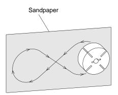
Figure 18 - Sanding Rotor
